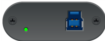
A flashing green LED means USB 2.0
