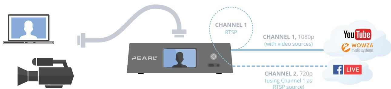
Figure 2 Using Pearl-2 with multi-streaming and multi-encoding
